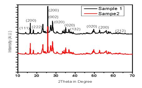
Fig. 1 X-ray diffraction pattern for WO<sub>3</sub> sample 1 and sample 2 at 120<sup>0</sup> C for 12 hours
