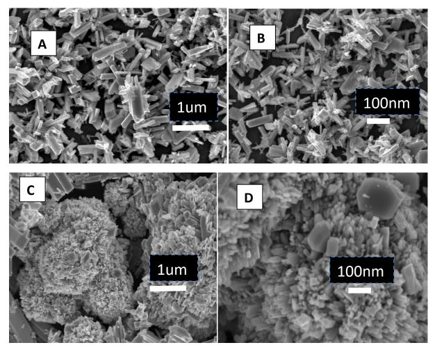
Fig. 2 FESEM image for WO3 film Sample 1 (A,B) and Sample 2 (C, D)
